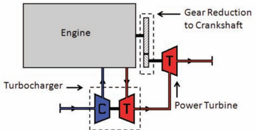
**FIGURE 3** Electric turbocompound on a turbocharged engine
