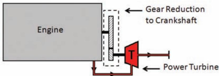
**RIGHT** Ready to move out of the dark ages? F1's engine technology has stagnated under the FIA's engine freeze. The 2013 season offers the opportunity to embrace solutions like turbocompounding
