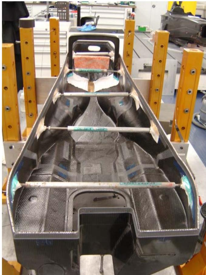
Figure 3. carbon composite/honeycomb chassis construction
