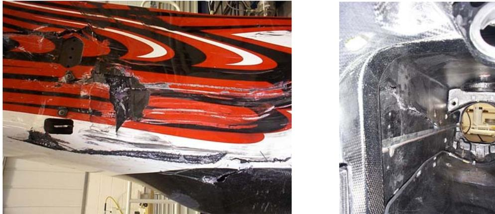
Figure 1. Penetration of the survival cell by a broken wishbone, resulting in injury to the driver’s leg.
