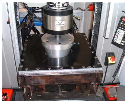
Figure 2. Intrusion panel test set-up.
