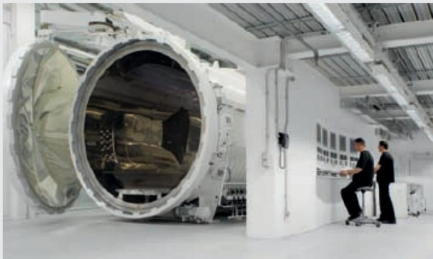
McLaren's autoclave facility at Woking produces moulded carbon fibre/aluminium honeycomb composites. In 2008 McLaren produced six chassis, in the 2009 season the number has been reduced to five due to testing restrictions. Each chassis takes approximately five weeks work, with teams working around the clock to finish © www.mclaren.com
