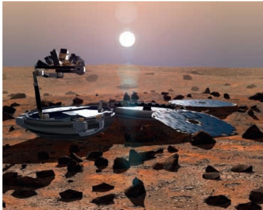
Beagle 2's outer skin was made of Kevlar, also used in Formula One racing since the 1970s and found in anything from the car's bodywork to the driver's safety clothing. The material is extremely heat resistant and can also remain strong at temperatures down to  $-196^{\circ}\text{C}$ , making it suitable for protecting the equipment from the freezing on Martian surface
