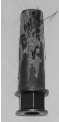
Figure 12 Fatigue failure in metal to composite joint
