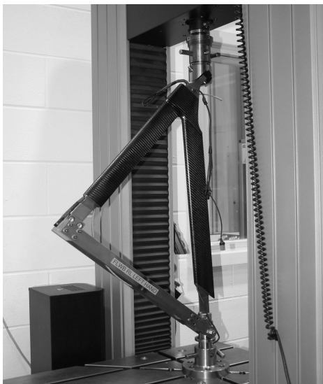
Figure 14. Proof testing a bonded composite wishbone
