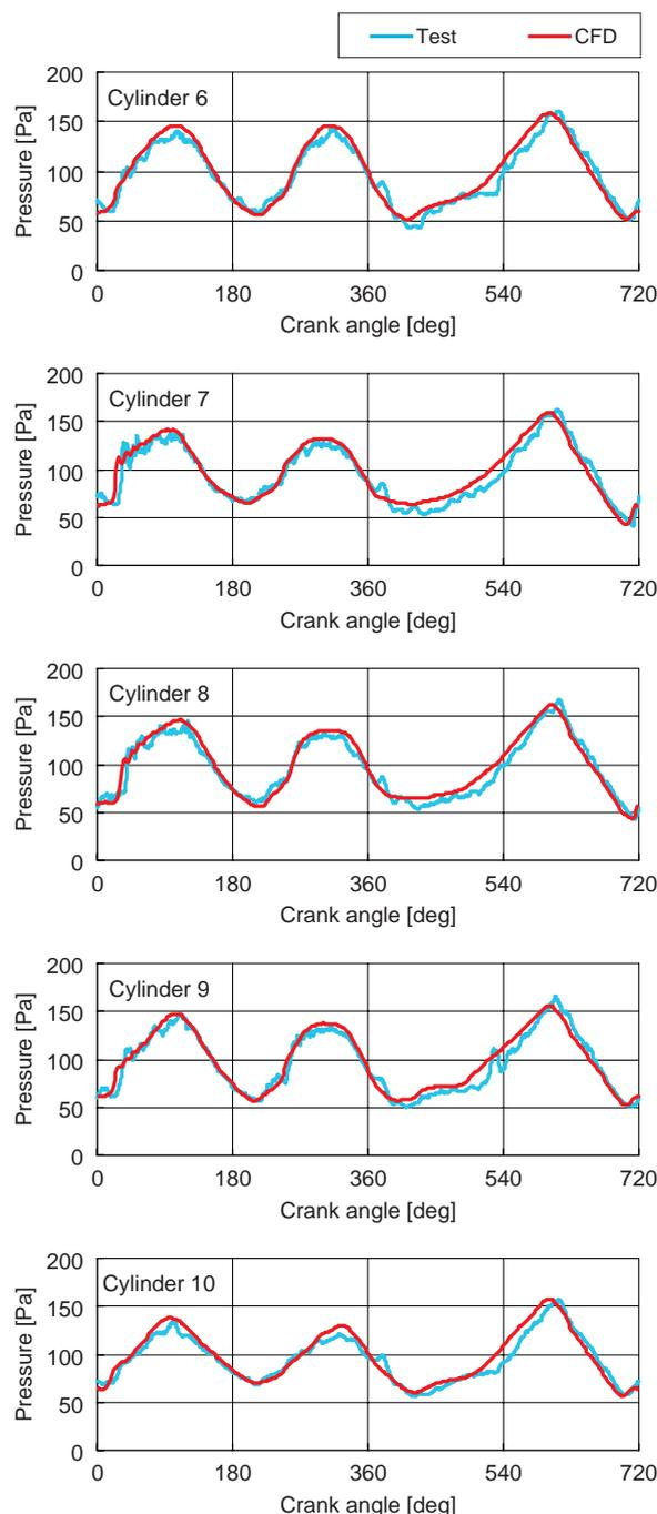
Fig. 2 Intake pressure of V10 engine at 17000 rpm
