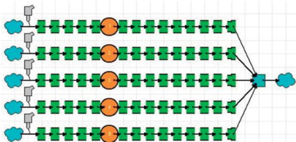
Fig. 4 WAVE model of 5 cylinders for V10 engine
