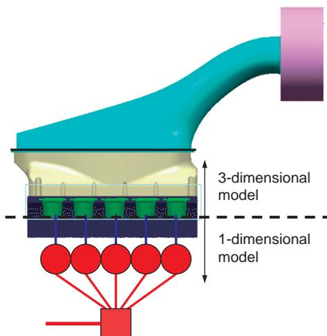
Fig. 1 Simulation model
