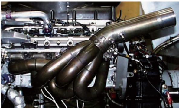
Fig. 3 Exhaust pipe of V10 engine
