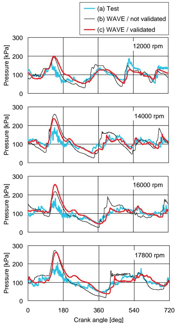
Fig. 5 Exhaust pressure of V10 engine (#10 cylinder)
